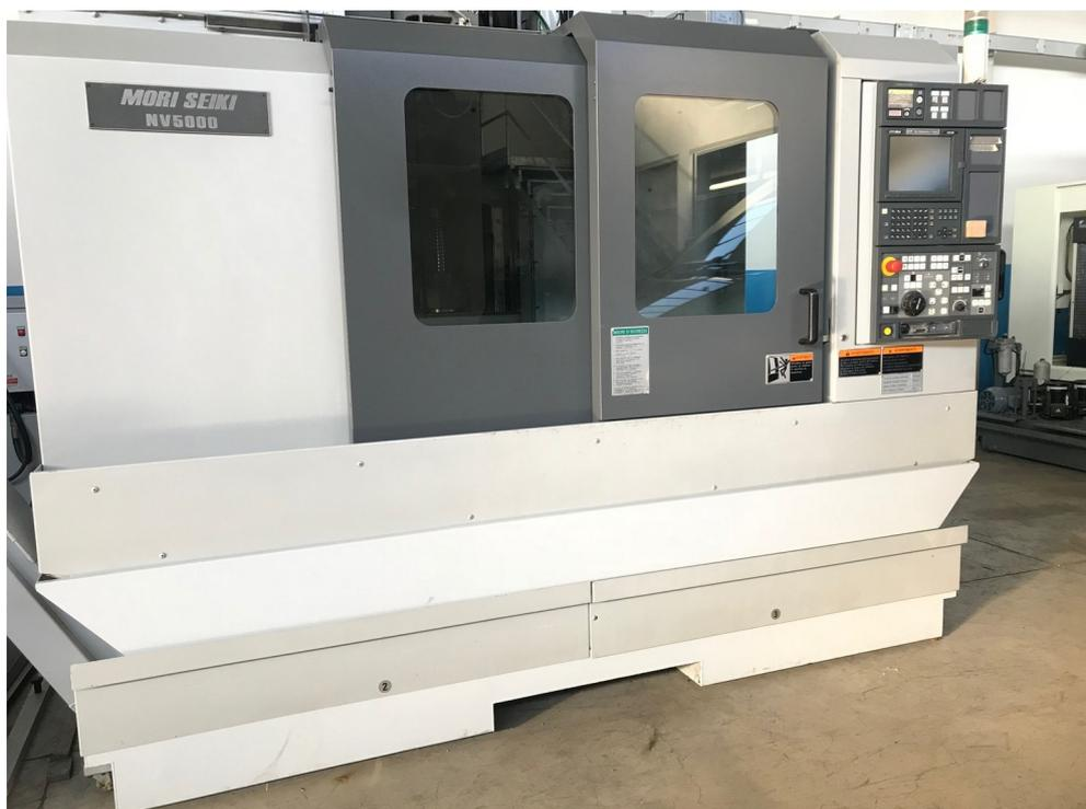
Controllo CNC: Fanuc MAPPS MSG-511
